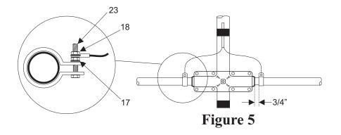
Attach the feed line to the driven element as shown in figure 5. Place the 5/8 clamps 3/4 inch away from the insulator. Use the 10-24 bolts nuts and lock washers to tighten the clamps to the tube. Place the feed line eyelets over the remaining section of the bolt and secure with another lock washer and nut. Secure the coax to the boom with electrical tape or other suitable fasteners.
