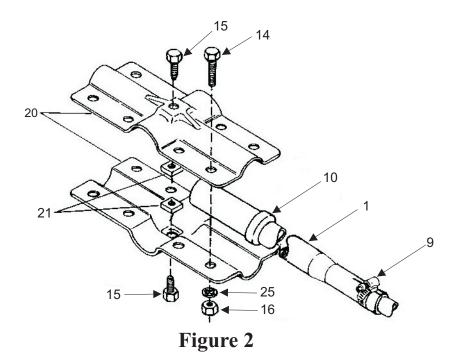
Secure the driven element insulator to the other end of the boom also allowing 3 inches from the center of the bracket to the end of the boom. Install the remaining two main elements to the insulator as shown in figure 2. Leave the bracket loose enough to align
