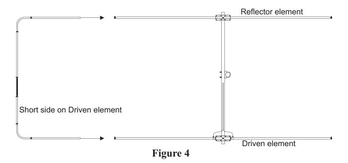
Install the end pieces onto the elements using the #4 hose clamps. Sliding these end pieces in and out will be how you adjust the final length of each element. Measure the distance from the center of the boom to the outside of the element. This distance will be the same for all four elements. Use the antenna diagram on the next page to verify all your measurements. Install the u-bolt on the boom. Place the 1-1/4 end caps on each end of the boom.
